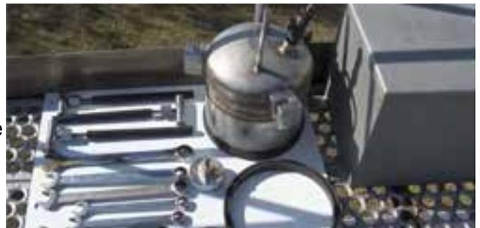
The Capping Kit components and required tools are stored in a weather-resistant, stainless steel box conveniently located on the upper platform of each Anhydrous HF trailer
